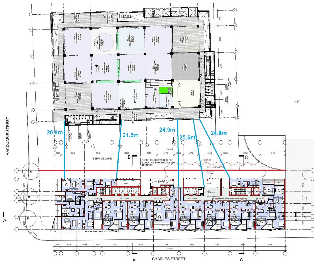
Figure 2. Separation between Level 8 of the school building (top) and Level 8 of the proposal (bottom).
